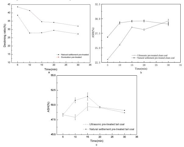
Fig. 2. Ultrasonic pre-treatment and natural sedimentation pre-treatment ash and deslimation rate (a: deslimation rate; b: the ash content of pre-treated clean coal; c: the ash content of pre-treated tail coal)
